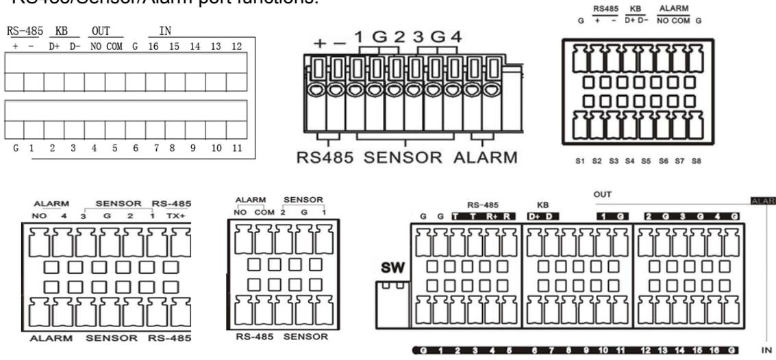
**Alarm input:** Connect [-] port of your sensor to G (GND) pin, and [+] port to channel input according to the alarm device you purchased.
