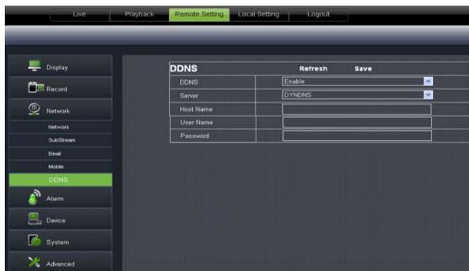
After user applies for DDNS service shown as Picture 6-24, you could enable <DDNS> function under any one network type mode (Static, DHCP and PPPoE). Now you remotely visit the DVR through domain name (<http://domain name: port No>). Details setting should be consistent with DVR local setting.
